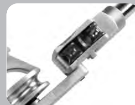
Roll Dies Reduce Force and Tube Flattening
