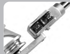
Roll Dies Reduce Force and Tube Flattening
