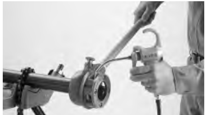
Figure 4 – Applying Thread Cutter Oil
