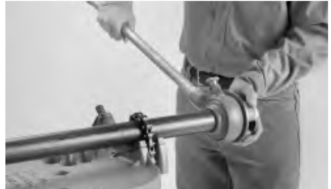
Figure 3 – Sliding Threader On Pipe
