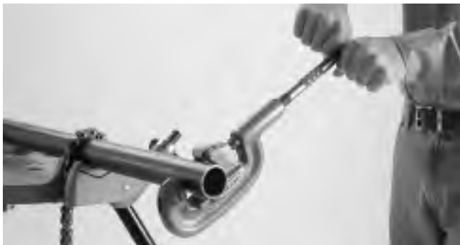
Figure 1 – Cutting End of Pipe
