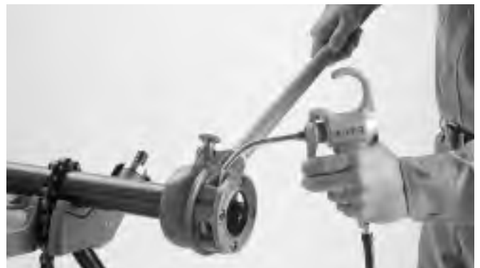
Figure 4 – Applying Thread Cutter Oil
