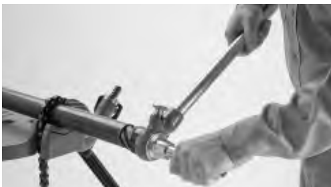
Figure 2 – Reaming End of Pipe
