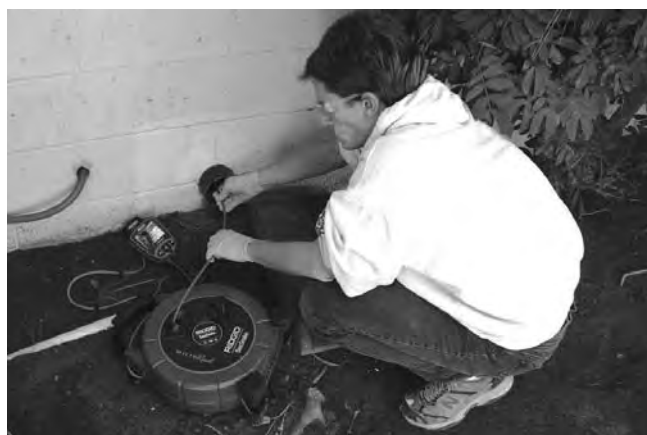
Figure 21 – Using The microReel
