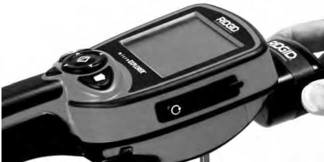
Figure 14 – Connecting the microEXPLORER Camera Monitor
