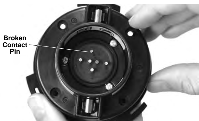
Figure 12 – Broken Contact Pin
