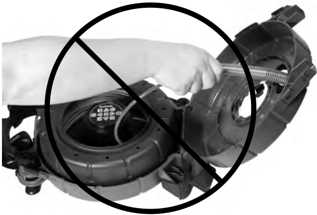
Figure 6 – Do Not Open Case Completely
