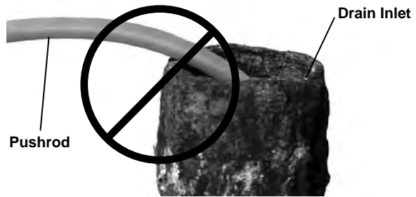
Figure 23 – Avoid Pulling At Sharp Angles
