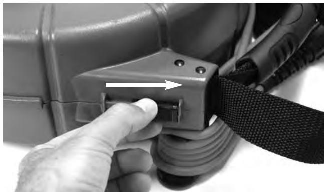
Figure 4 – Unlatching the microReel Case
