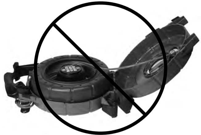
Figure 9 – Do Not Open Case with Camera Outside
