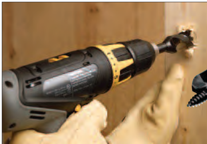
Mini™-Augers are an excellent choice for working in tight spaces.
