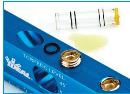
2. Remove O-ring and damaged vial
