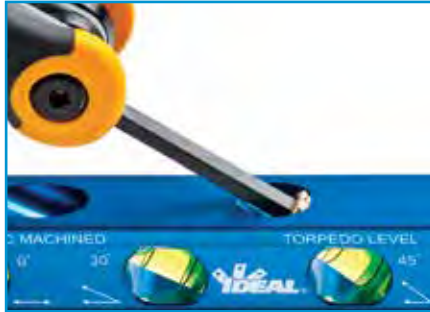
1. Remove the set screw with hex wrench
