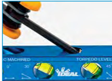
4. Reinstall O-ring and set screw
