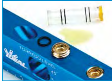
2. Remove O-ring and damaged vial
