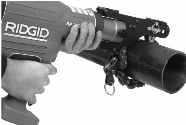
Figure 5 – Cutting The Pipe
