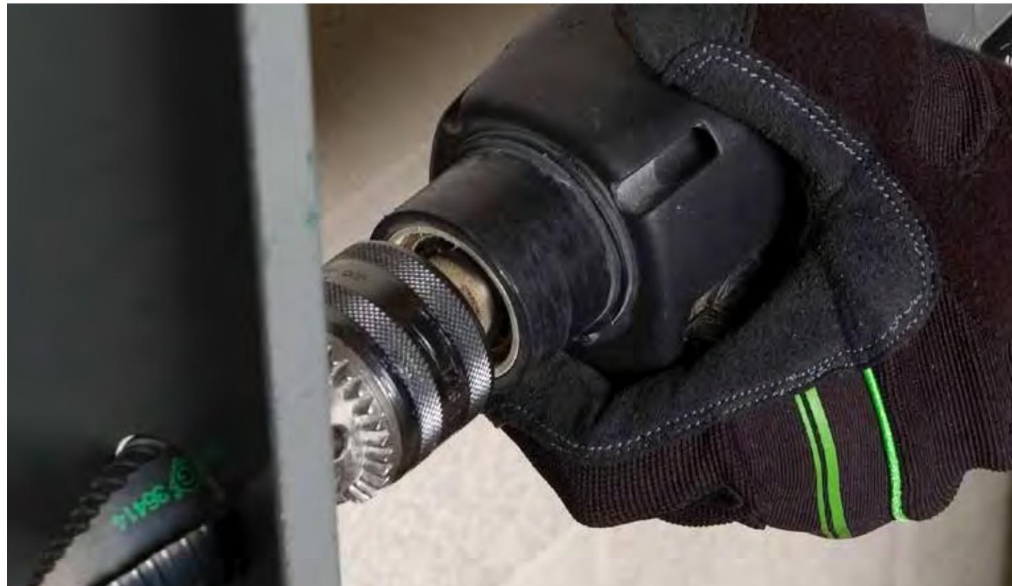
Single-hole bits are designed to drill one indicated hole size through a series of steps from bit tip to full size
