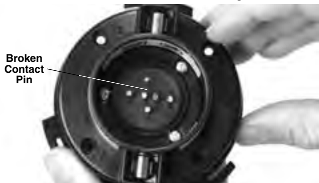
Figure 7 – Broken Contact Pin
