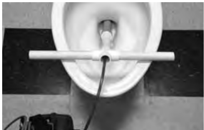
Figure 24 – Using A PVC Guide Tube
