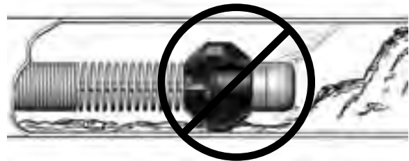
Figure 17 – Encountering An Obstruction – Do Not Use Camera Head To Clear Obstructions
