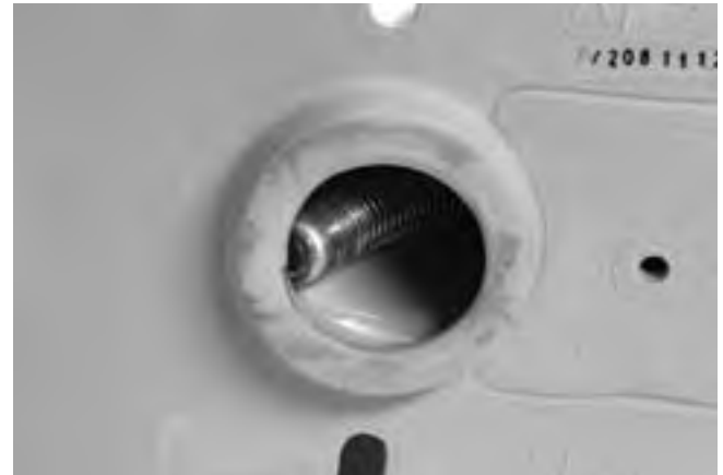
Figure 20 – Camera Head Blocked in Turn
