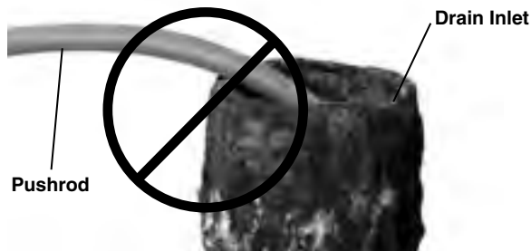
Figure 18 – Avoid Pulling At Sharp Angles
