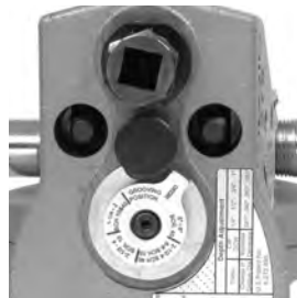
Figure 5 – Gauge In Grooving Position
