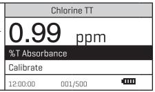
11. Press or to scroll to the concentration of the standard, 1.00 in this example. Note: The allowable adjustment is ±25%.
