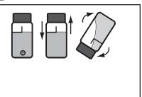
NOTE: For wastewater samples, **Standard Methods for the Examination of Water and** Wastewater recommends waiting 2 minutes for full color development when testing total chlorine.
