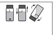
Immediately insert tube into chamber, Close lid, Select Scan Sample. Record result as Bromine.
