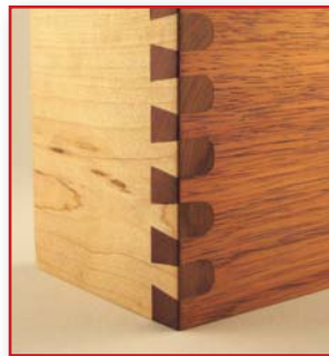
Cuts Through Joints
