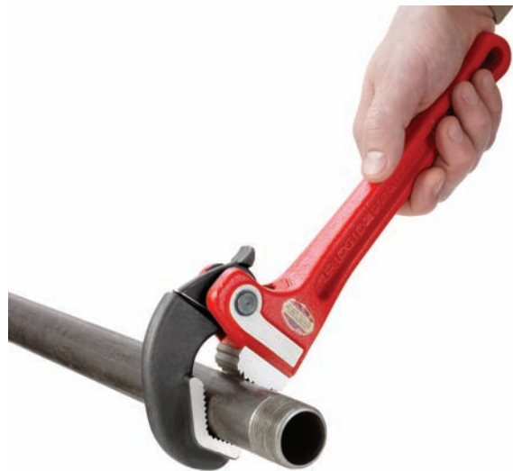
Figure 5 – Using a RapidGrip Wrench
