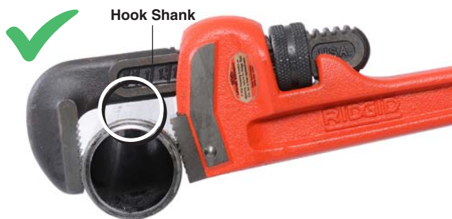
Figure 3 – Maintain Gap Between Hook Shank and Work Piece
