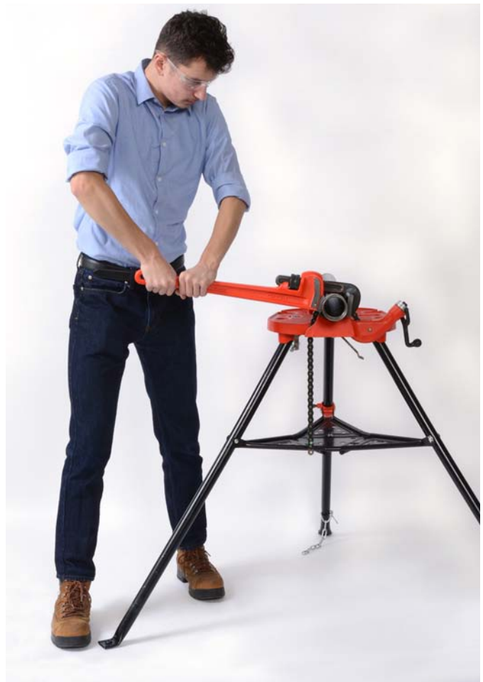
Figure 7 – A Proper Operating Position
