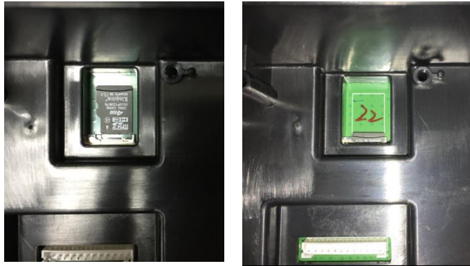
Figure 2-5 Sliding an SD Card into the SD Socket (left); SD Card Installed (right)
