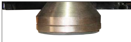
Stainless steel feet with rubber bottoms are attached to each load cell – ball-in-cup design makes feet self-swiveling and base easier to level
