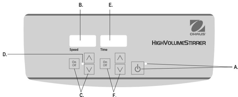
The front panel of the High Volume Stirrer - STHVDG contains all the controls and displays needed to operate the unit.
