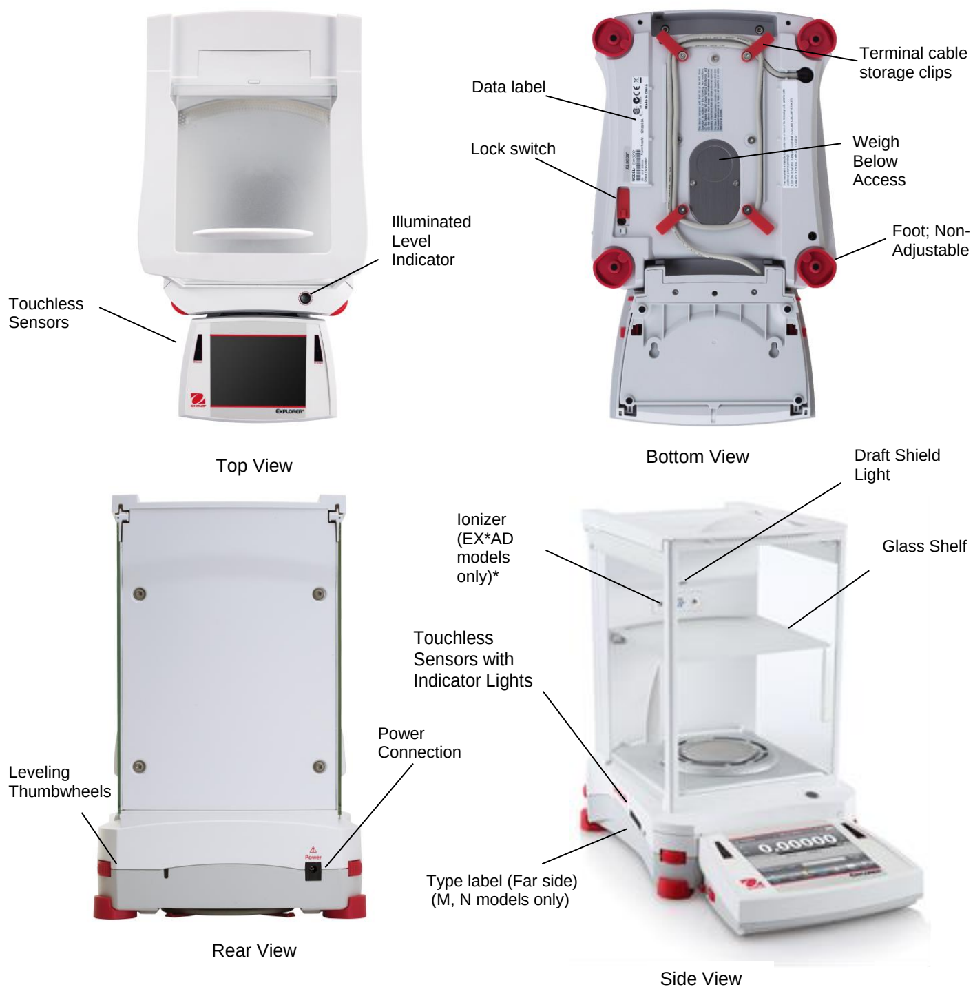
Figure 3-1. Explorer Semi-Micro Balance
