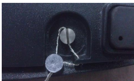
Locked with Wire Seal
