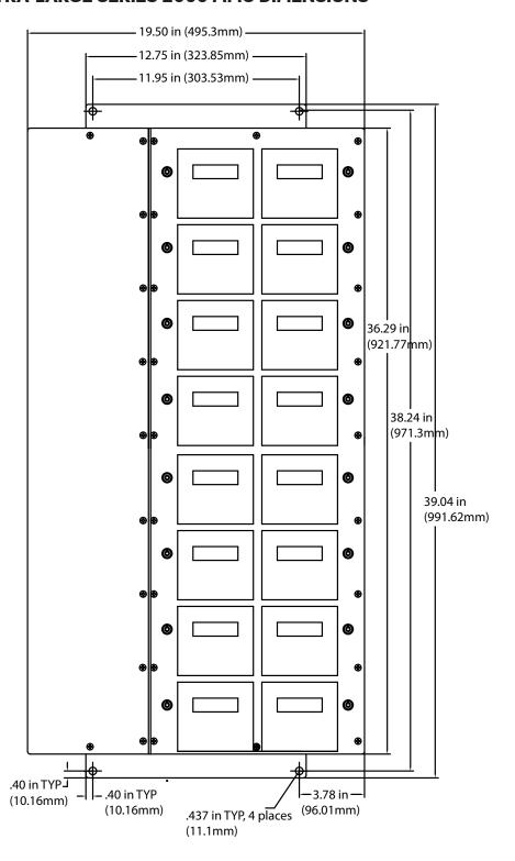
NOTE: Overall depth of all MMU enclosures is 3.85 in (97.79mm).
