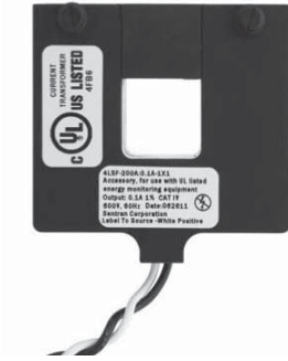
Figure 6: Leviton split core CTs
