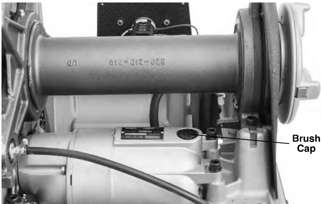
Figure 34 – Removing Motor Cover/Changing Brushes
