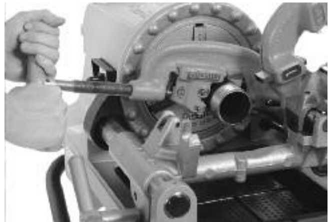
Figure 22 – Cutting Pipe with Cutter
