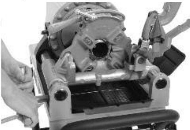
Figure 24 – Threading Pipe (811-A Quick Opening Die Head shown)
