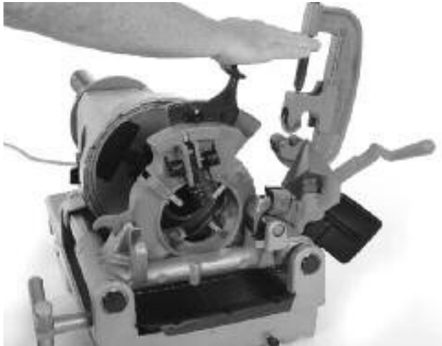
Figure 19 – Closing the Receding Die Head
