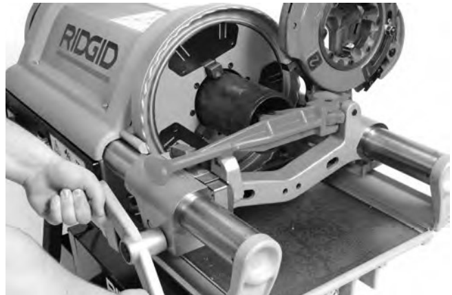
Figure 22 – Reaming Pipe with Reamer
