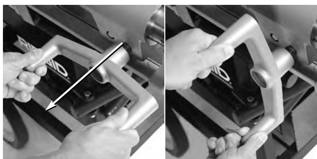
Figure 20 – Carriage Handwheel Adjustment
