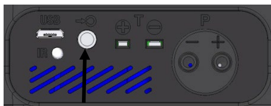
Fig. 45: Connectors for the wood moisture probe at the bottom of the analyzer
