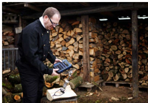
Fig. 46: Wood moisture measurement with Probe Wohler HBF 420.
