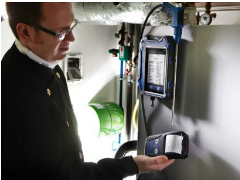
Fig. 35: Printing the readings of the Wohler A 550 INDUSTRIAL on the Ther-moprinter Wohler TD 100.
