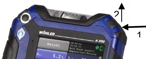
Fig. 67: Open the condensate trap compartment
