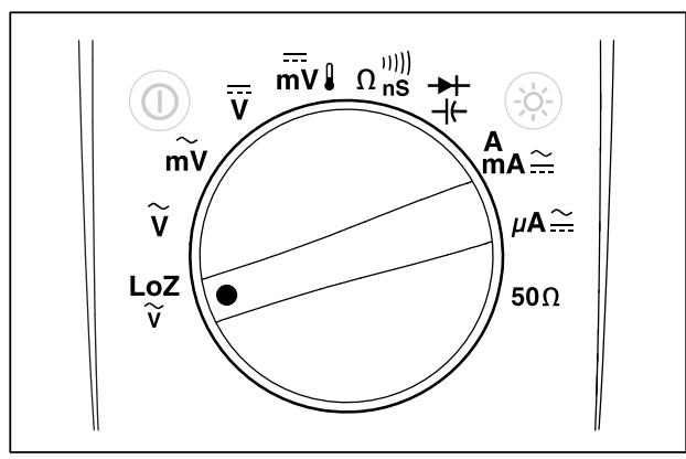
Figure 3. Rotary Switch
