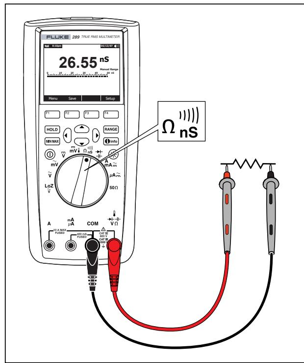
Figure 18. Conductance Measurement
