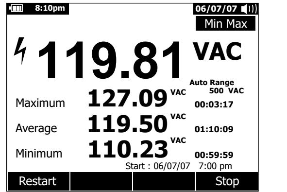
Figure 6. MIN MAX Record Display
