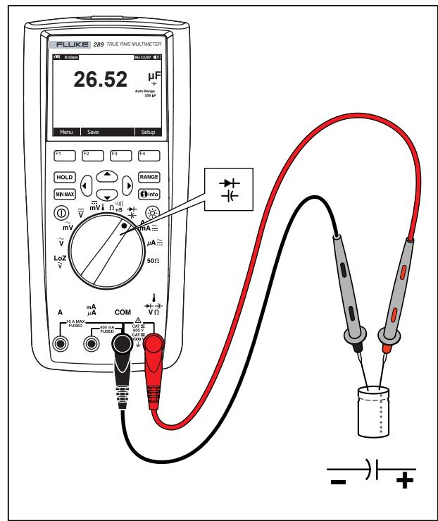
**Figure 19. Capacitance Measurement**
