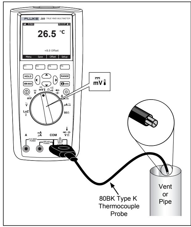
Figure 14. Temperature Measurement
