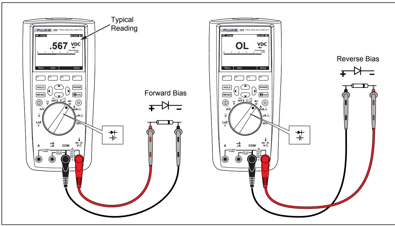
**Figure 20. Diode Testing**
