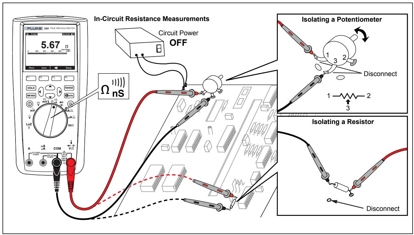
Figure 15. Resistance Measurement
