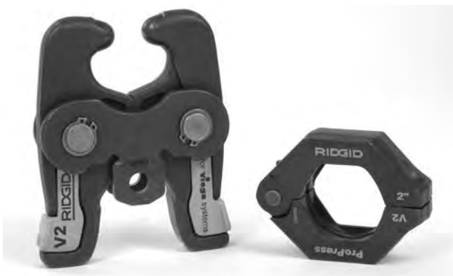
Figure 3 – ProPress Ring and V2 Actuator
