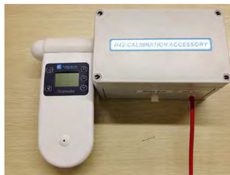
Use this orientation for calibrating CO
