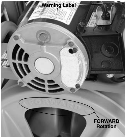
Figure 8 – Proper Drum Rotation (FOR Switch Position)
