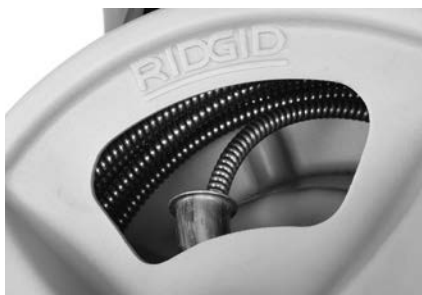
Figure 18 – Coil Cable Into Drum As Shown
