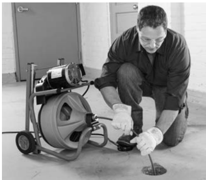
Figure 13 – In Operating Position, Manually Feeding Cable
