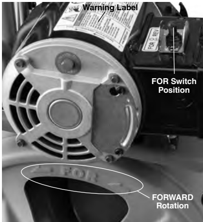
Figure 8 – Proper Drum Rotation (FOR Switch Position)
