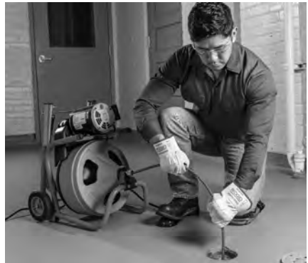
Figure 13 – In Operating Position, Manually Feeding Cable
