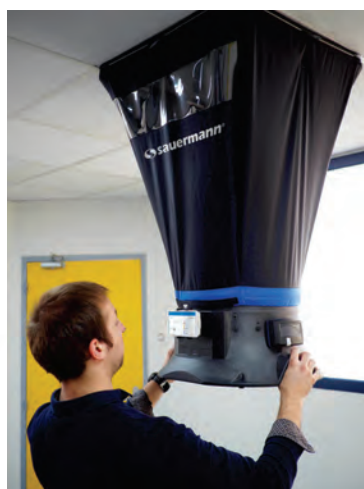
Use of the air flow meter
