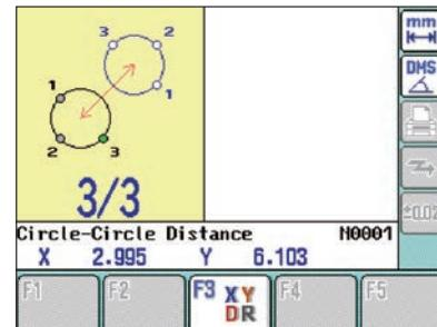
2. Determine each position (a1, a2, a3) on round hole A, following the measurement navigation procedure on the LCD.
