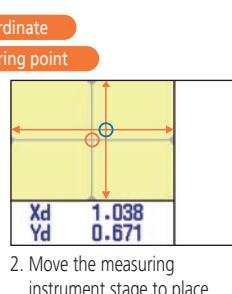
2. Move the measuring instrument stage to place one set of cross-hairs over the other (or to bring the counter reading to zero).
