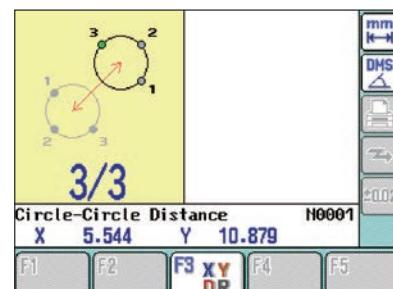
3. Next, the measurement navigation procedure for round hole B will be displayed. Determine each position (b1, b2, b3) in the same manner as in step (2).
