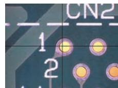
4. Press [LOAD] to enter data, using the cross-hairs of the measuring instrument.
