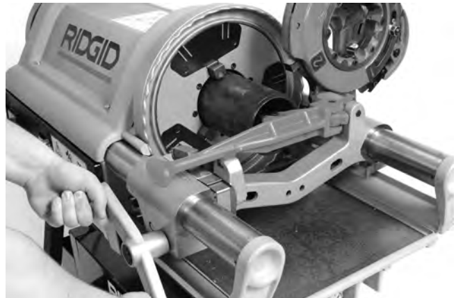
Figure 22 – Reaming Pipe with Reamer
