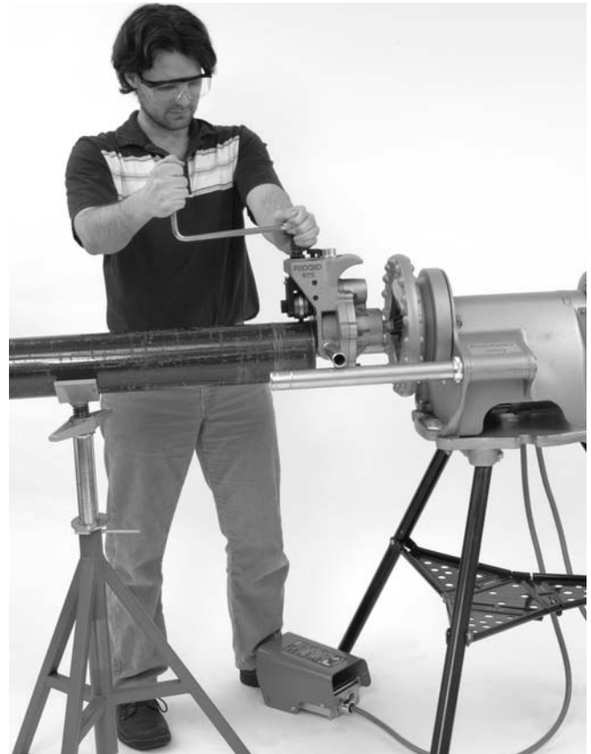
Figure 12 – Roll Groover Operating Position
