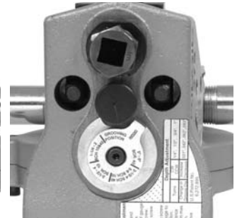
Figure 15B – Gauge In Grooving Position
