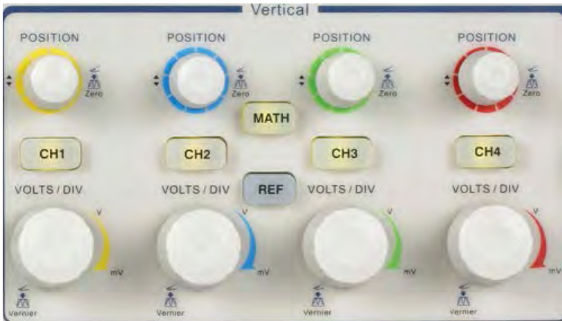
Figure 15 - Vertical System Controls
