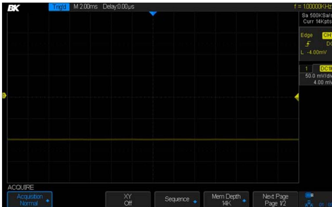
Figure 34 - Pulse with 0.1% duty cycle, normal mode
