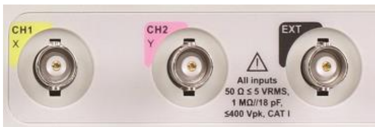
Figure 15 - Analog and external trigger connectors
