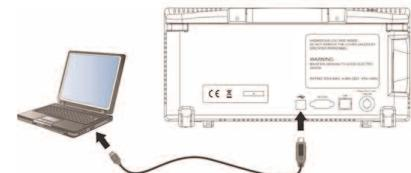
Remotely connect to the scope and download waveform data from custom software using SCPI commands.
