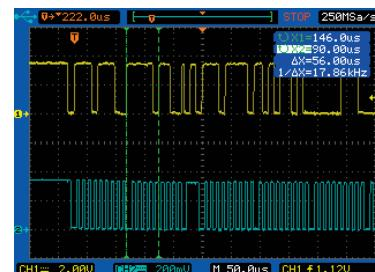
Beneficial for applications such as I<sup>2</sup>C serial data streams, deep memory lets you capture waveforms in high resolution while maintaining a high sample rate over a longer period of time. Up to 2.4 Mpts of memory can be captured in as fast as 5 seconds\* using binary transfer through the LAN or USB interface.
