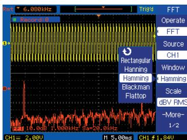
Display and measure the input signal's frequency spectrum. Select one of the 5 FFT windows: Rectangular, Hanning, Hamming, Blackman, and Flattop. Use cursors to measure the spectral component's magnitude and frequency.
