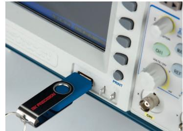
Save and load arbitrary waveform data in CSV format from a USB flash drive.
