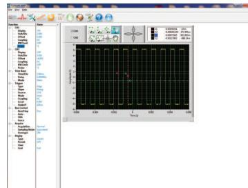
Comsoft software provides seamless integration between the oscilloscope and PC. Capture and transfer waveforms, screen images, setups, and measurement results to a Windows PC via the LAN and USB device port on the back of the instrument. A USB host port on the front allows for quick and easy screen saving to a USB flash drive.
