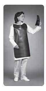
This Beta-Blocking neoprene apron (1/8" thick) blocks up to 96% of the high energy beta rays from Strontium-90 and over 98% of the beta rays from Phosphorous-32.
