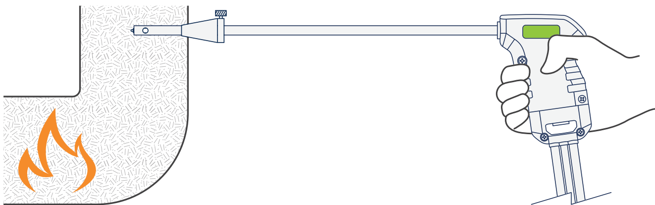
Fig. 3-6: Probe Placed in Center of Measurement Area
