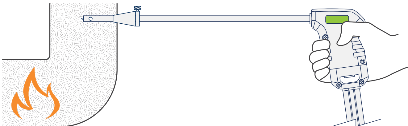
Fig. 3-6: Probe Placed in Center of Measurement Area
