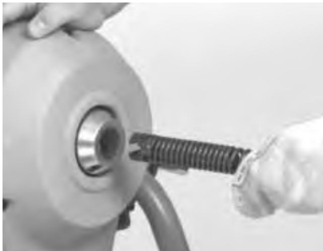
Figure 4 – Inserting Cable Into Front Of Machine
