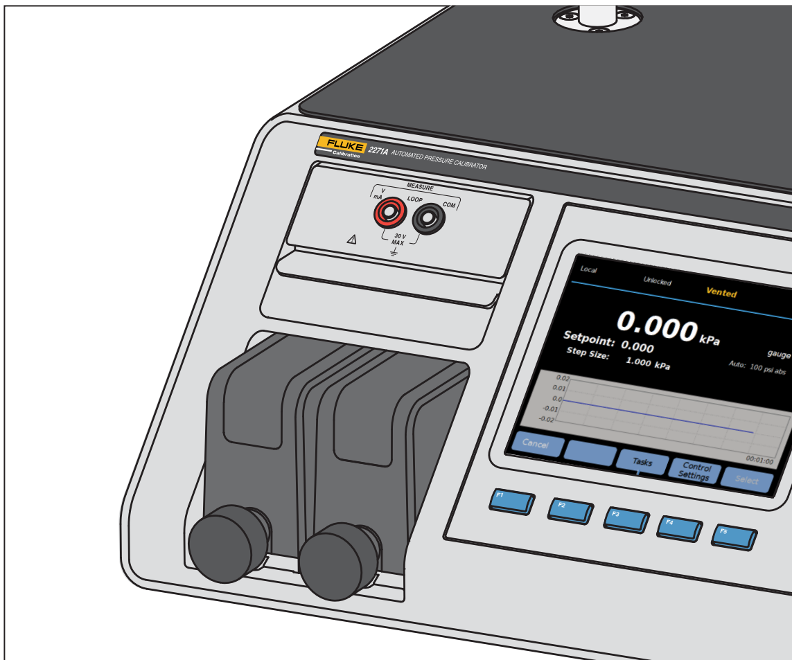
Figure 3. Installed EMM and PMM Modules
