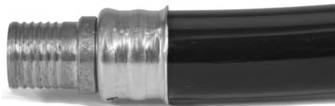
Figure 3 – Completed Pressed Fitting
