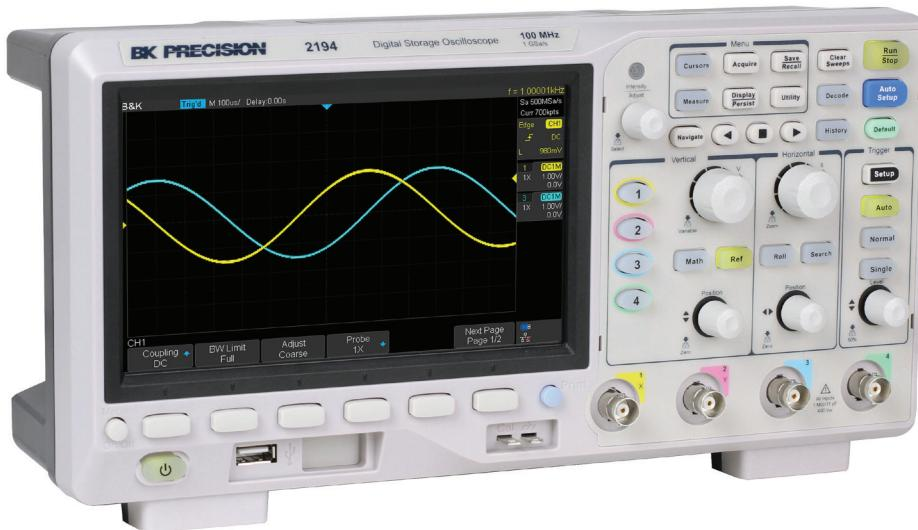
The 2194 combines performance and value all in one portable solution. This oscilloscope provides 100 MHz of bandwidth in a 4-channel configuration with a maximum sample rate of 1 GSa/s and a maximum memory depth of 14 Mpts. Equipped with a 7" LCD display and a waveform update rate of 100,000 waveforms per second, this device is able to capture infrequent glitches with excellent signal fidelity.
