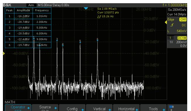
Displays signal in the frequency domain to ease measuring wave harmonics or discovering applications potential noise induced by frequency dependent components.
