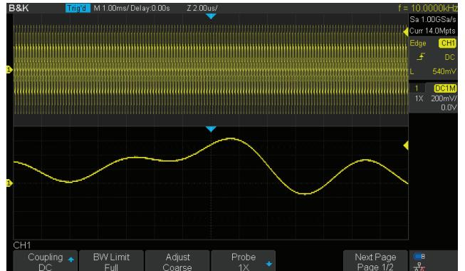
Capture longer time periods at higher resolution with a maximum memory depth of 14 Mpts. Enable zoom feature to display specific events in more detail.
