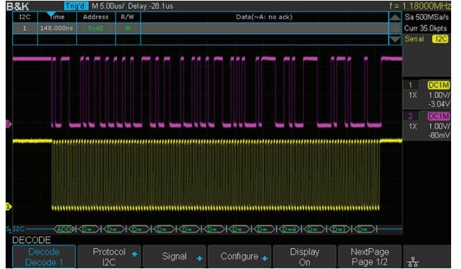
Serial bus decoding supports I<sup>2</sup>C, SPI, UART, CAN and LIN protocols. Information can be quickly displayed in a tabular format.
