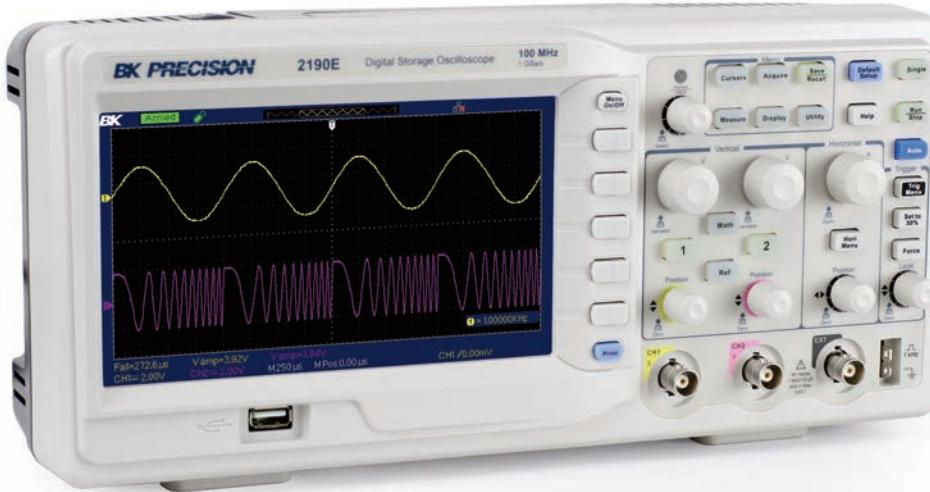
The 2190E combines performance and value all in one portable solution. With 100 MHz bandwidth and 1 GSa/s sample rate, these oscilloscopes offer advanced triggering capabilities, long waveform memory up to 40,000 points, and extensive features such as pass/fail limit testing, digital filtering, waveform recorder, and 32 automatic measurements.
