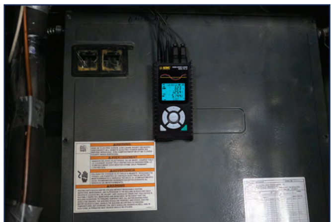
In this study, the load analysis was conducted using the AEMC® Instruments PEL 52. To secure the device in place during the week-long testing period, four powerful magnets on the casing allow it to be easily attached to the flat metallic surface of the HVAC system.
