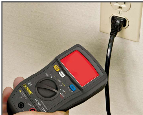
Non-contact detection of network voltage (NCV Function-AC only)
